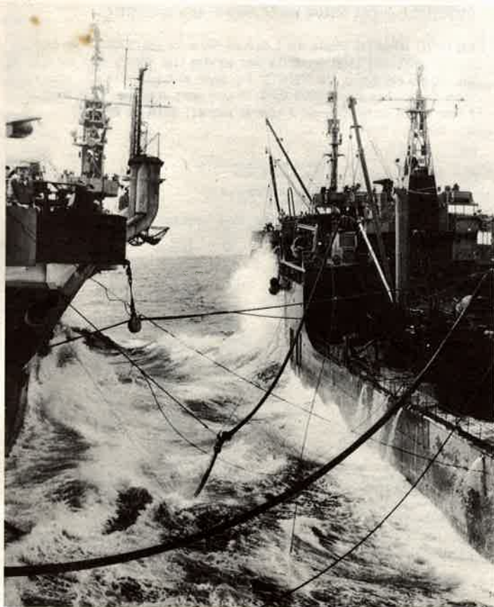
Water breaks high on the sides of an Esso tanker as she pumps fuel to a light carrier in one of the many fueling-at sea operations that made long range strikes against the enemy possible. When this picture was taken, heavy swells had brought the two ships close together. Slack on the hose astern had been taken up smartly, but the hose forward still is dragging in the water. August 11, 1945.
